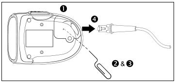
Figure 7. Releasing the PowerLink Cable
