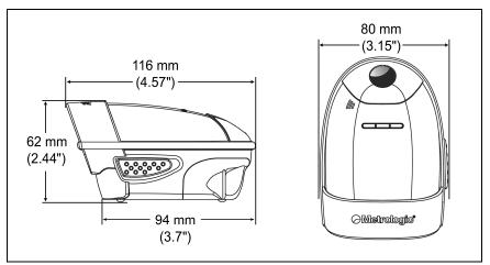
Figure 2. Scanner Dimensions
