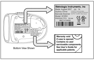
Figure 4. Label Samples and Location
