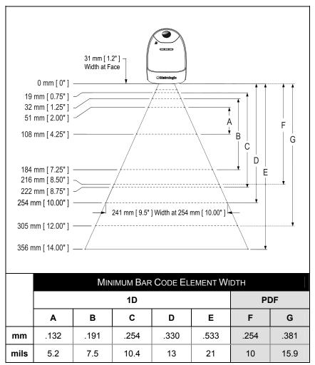
Figure 17. Depth of Field by Minimum Bar Code Element Width
