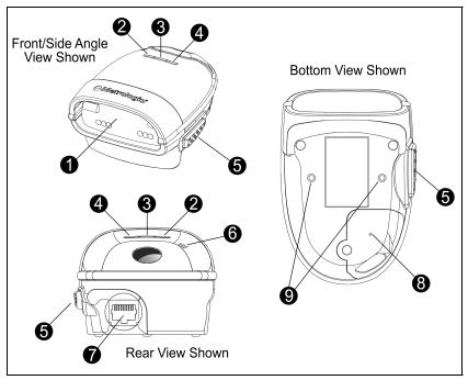
Figure 1. Scanner Components
