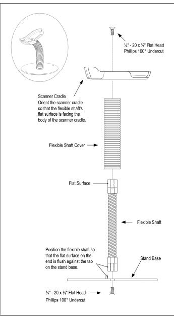
Figure 14. Assembling the Stand
