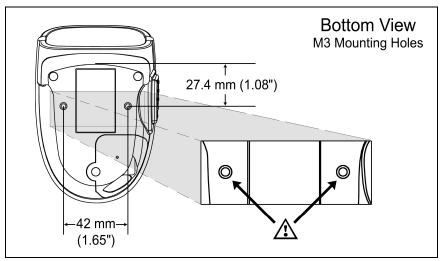
Figure 3. M3 Mounting Hole Dimensions
