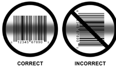
Figure 18. 1D Bar Code Orientation
