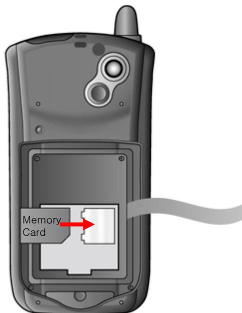
\* Push the memory card into the slot as shown until it's plugged.
