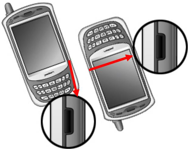
• Matching the IrDA port as shown (transmission speed is fastest when the distance at shortest)
