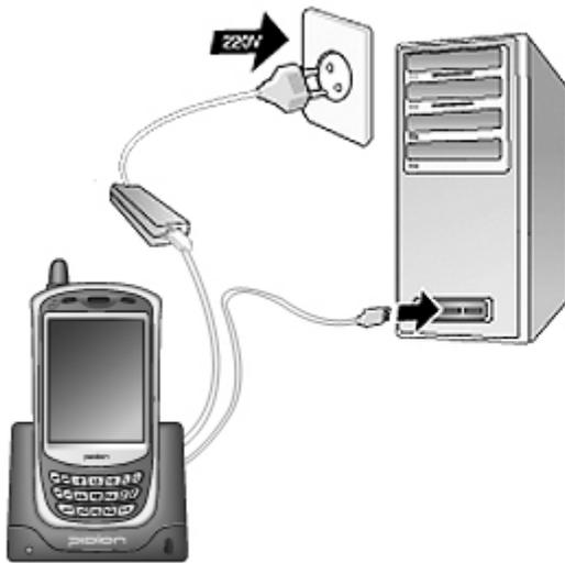
\* Connect the PDA (cradle) -cable-computer as shown
