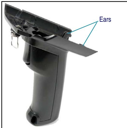
2. Seat the top of the Handle against the Pegaso and turn the quarter-turn fastener to secure the Handle to the unit.
