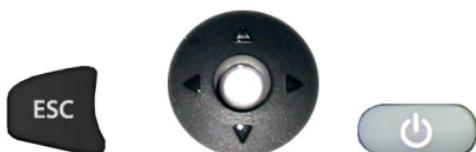
By pressing ESC + JOYSTICK select + ON/OFF keys simultaneously, a system hardware reset is performed.
