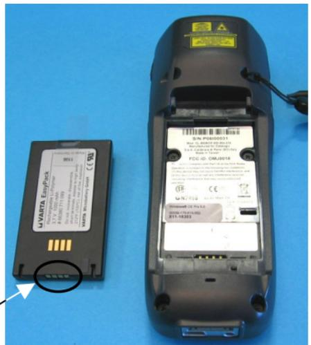
4. Install the new battery pack, first insert the bottom (contacts) side, then the upper (lock) side as indicated in the following figure:
