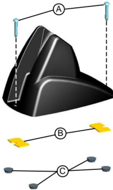
The stand can be mounted by using self-tapping screws, double sided adhesive strips or rubber feet:
