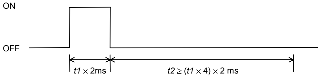
Figure F-1 Drawer Drive Signal Waveform (Formulas F-1 and F-2)
